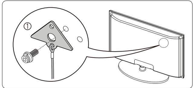
2. Firmly fasten the screw you provided (size M4xL20 or similar) to the wall or cabinet where the TV is to be installed.
