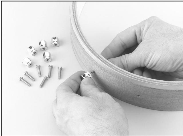
**Figure 4.** Installing the bracket hook lugs.
