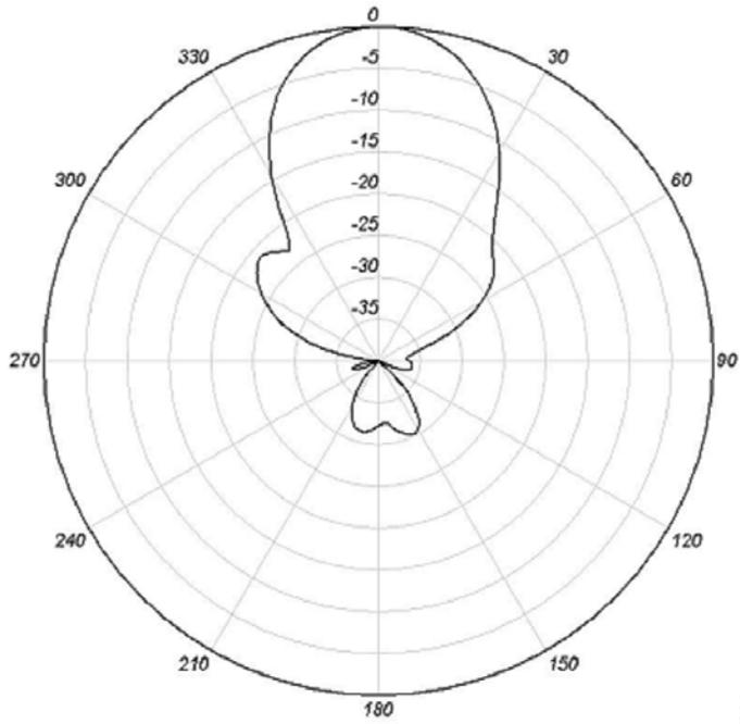
2.4 GHz Ports A&C Elevation Plane
