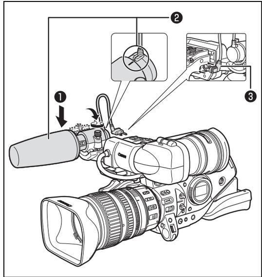
**i** To use an external microphone with a diameter too small for the microphone holder to close securely, attach first the supplied adjustment band to the microphone holder and then insert the microphone.
