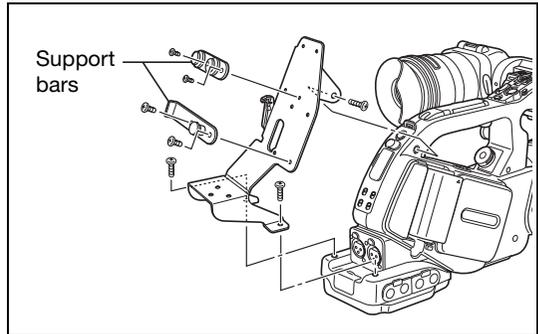
When using the optional CH-910, hook it onto the support bars and secure it with the stop lever. To detach the CH-910, press the stop lever in the direction of the arrow and pull the CH-910 off the support bars.
