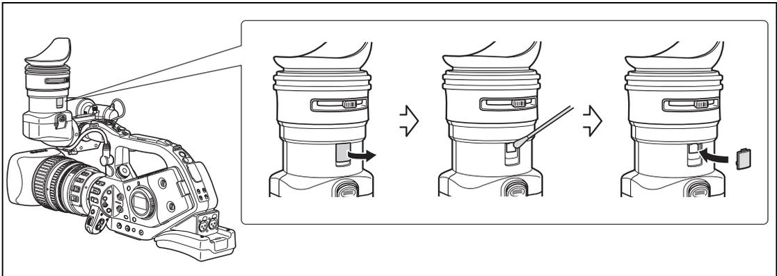
1. Open the protecting cover (e.g. using a flathead screwdriver).
