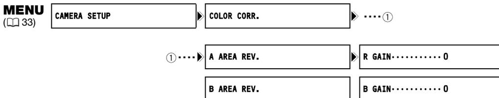
1. Open the menu and select **[CAMERA SETUP]**. Select the **[COLOR CORR.]** submenu and then select **[A AREA REV.]** or **[B AREA REV.]**.
