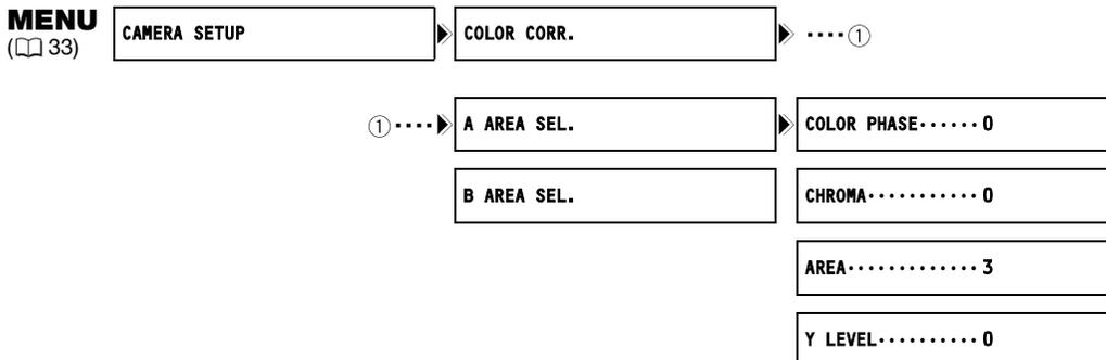
1. Open the menu and select **[CAMERA SETUP]**. Select the **[COLOR CORR.]** submenu and then select **[A AREA SEL.]** or **[B AREA SEL.]**.
