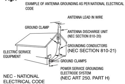
14. Lightning — For added protection of this product during a lightning storm, or when it is left unattended and unused for long periods of time, disconnect it from the wall outlet and disconnect the antenna. This will prevent damage to the product due to lightning and power-line surges.
