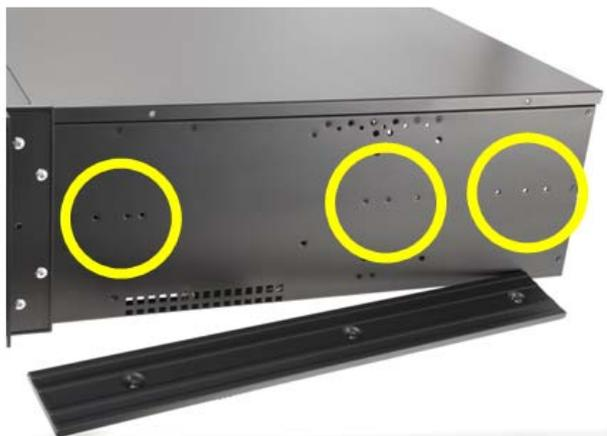
3. Upon removing the side bar, you will find several screw holes for you to install the server rail.
