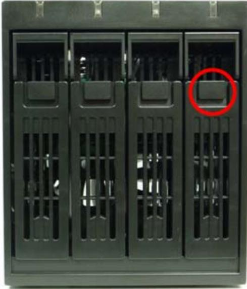
1. Each HDD Tray has a press button for releasing the hinge. To remove the HDD Tray; first press the button (red circle).
