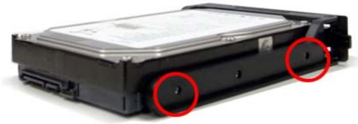
2. Once align, you can fasten the screws on both side of the tray to fix the HDD. (Please make sure that the connector of the HDD is facing outward)
