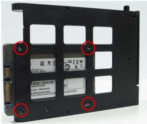
2. Once align, you can fasten the screws on the tray to fix the HDD. (Please make sure that the connector of the HDD is facing outward)
