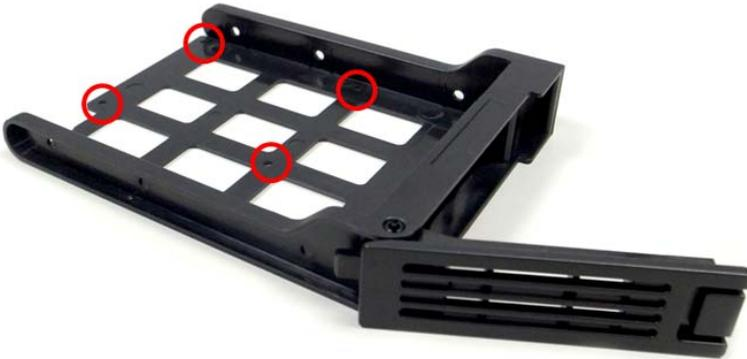
1. To install a 2.5" HDD, please make sure that the 2.5" HDD is align with the screw holes on the tray
