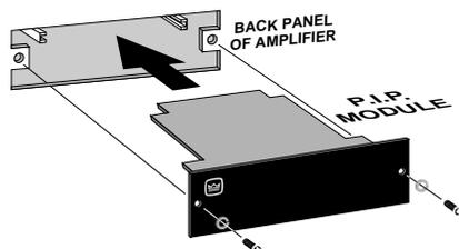
Fig. 3.3 Installation into a Standard P.I.P. Amplifier
