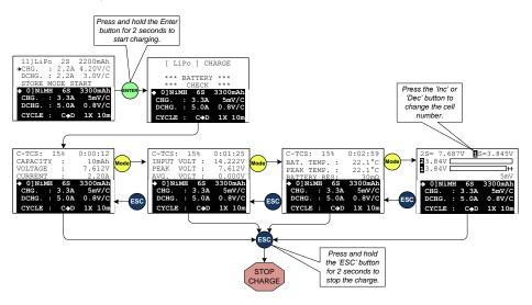
With the line selection arrow on the 'CHG.' line, check the correct charge current and cell voltage is selected, then press and hold the 'Enter' button for 2 seconds to start the charge.
