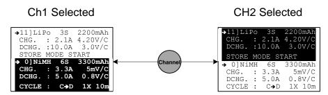
Pressing the 'Channel' button (at any time) selects the other channel (charger).
