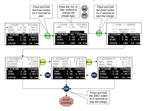
After selecting charge for a NiCd or NiMH pack, you are given the option to select four different charge types. These are:-
