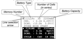
To edit the battery parameters, make sure the selection arrow is on the top line and press the 'Enter' button to highlight the memory number. Using the 'Inc' or 'Dec' buttons, the selected memory (0~19) can be changed. By default each memory is populated with a sample configuration, but these can be adjusted to suit your requirements.
