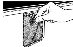
3. To replace, push the replacement filter into place. Insert the bottom tabs of the Air Filter Cover and push in until the side tabs snap into place.
