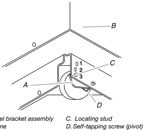
2. Use pliers to lower leveling legs away from cabinet. Adjust legs so there will be a  $\frac{1}{8}$ " (3 mm) to  $\frac{1}{4}$ " (6.4 mm) space between the top of the compactor and the top of the cabinet opening. Stand the compactor upright.
