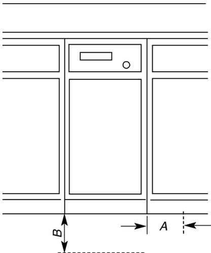
A. Leave 6" (15.2 cm) of clearance space to the right side of the compactator in order to remove the compactor bags.
