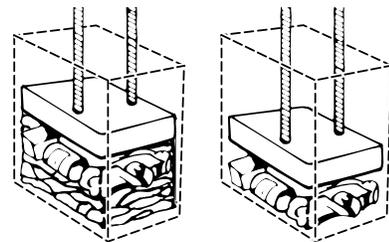
Load bulky trash, bottles, and cans in the center of the drawer. Bottles or cans not placed in the center may become caught between the ram and the drawer. The Drawer Monitor Switch then senses a "mismatch" and causes the ram to return to the "up" position without compacting.
