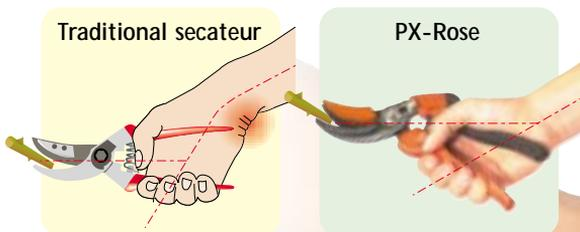
▶ The dual inclination of the cutting head compensates the wrist bending and allows the hand to remain in a neutral position
