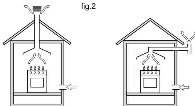
In a chimney stack or branched flue
