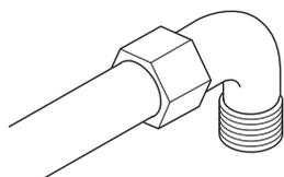
appliance to the right (fig.8), or flexible steel pipe in compliance with the standards in force, which must not exceed 2000 mm in length. Should it be necessary to turn the fitting, the gasket (supplied with the appliance) must be replaced.
