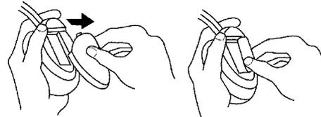
2. Turn the headphone volume nearly off before turning on the power. Turn on the headphone power then adjust the headphone volume louder to a comfortable level (You can adjust the audio source volume louder if needed, if connected to a variable audio source, such as a headphone source).
