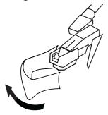
Turn the TURNTABLE SUSPENSION SCREW (28) clockwise until it is all the way down. Do not force or over tighten it. This allows the turntable to float on its shock absorbers.
