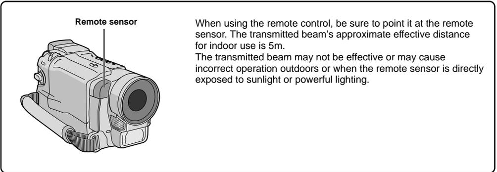
When using the remote control, be sure to point it at the remote sensor. The transmitted beam's approximate effective distance for indoor use is 5m.
