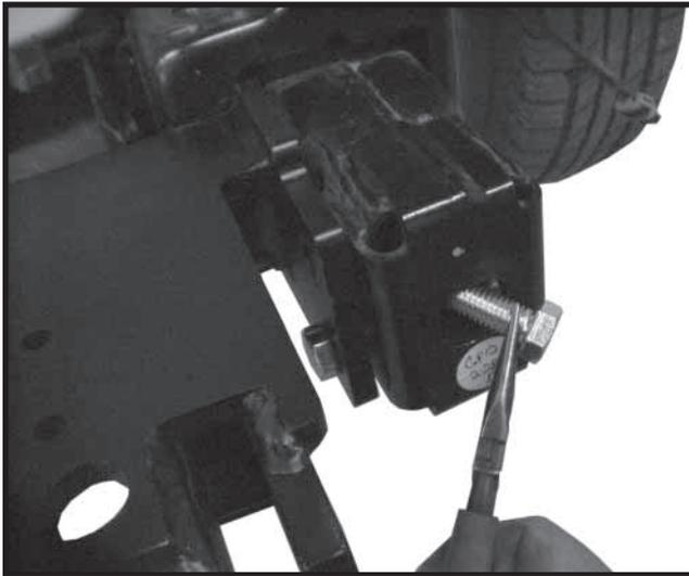
9. If drilling is needed insert shorter bolt using needle nose pliers as shown above.
