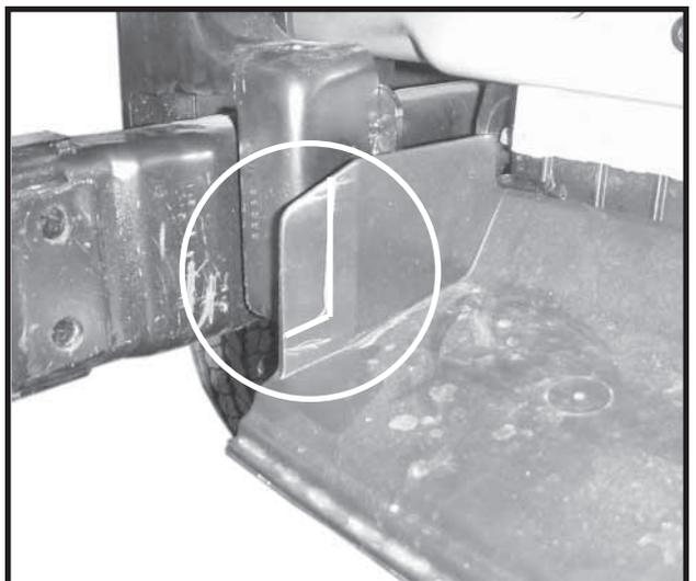
7. Notch plastic shield according to picture.
