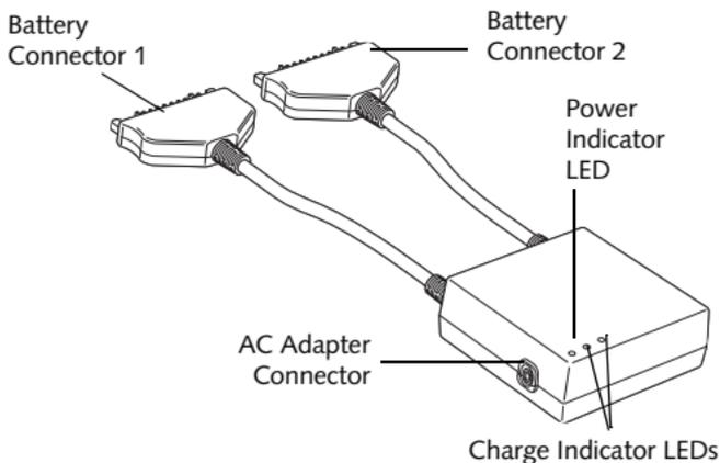
Figure 1. Battery Charger Components
