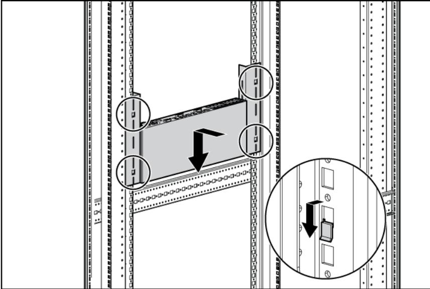
4. Install four cage nuts into the side-mounting bracket U locations.
