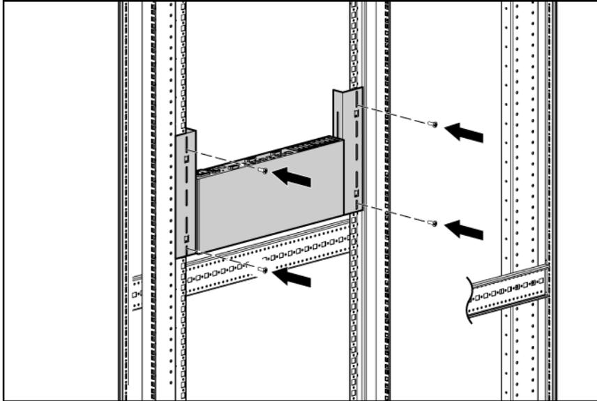
**NOTE:** Some racks enable you to use four sheet metal screws in place of M-6 screws and cage nuts.
