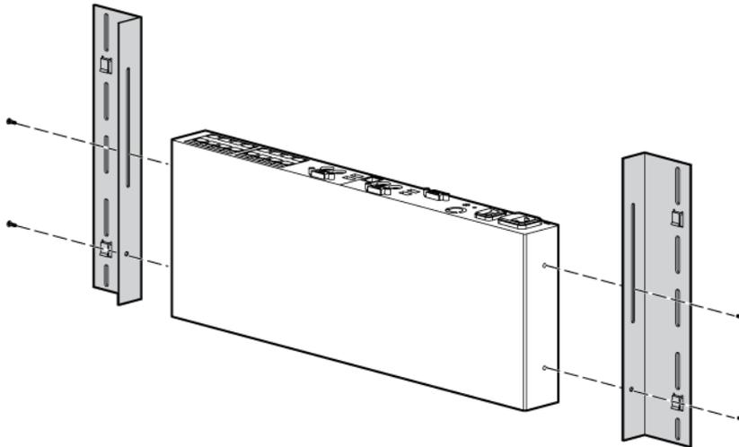
3. Slide the side-mounting bracket tabs into the U locations on each side of the rack.
