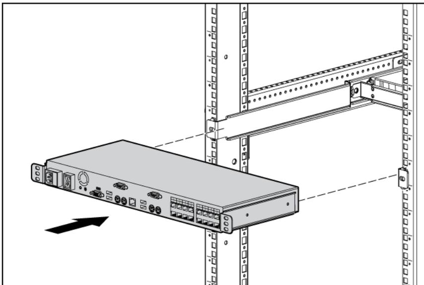
5. Secure the console switch to the rails using two M-6 screws, one on each side.
