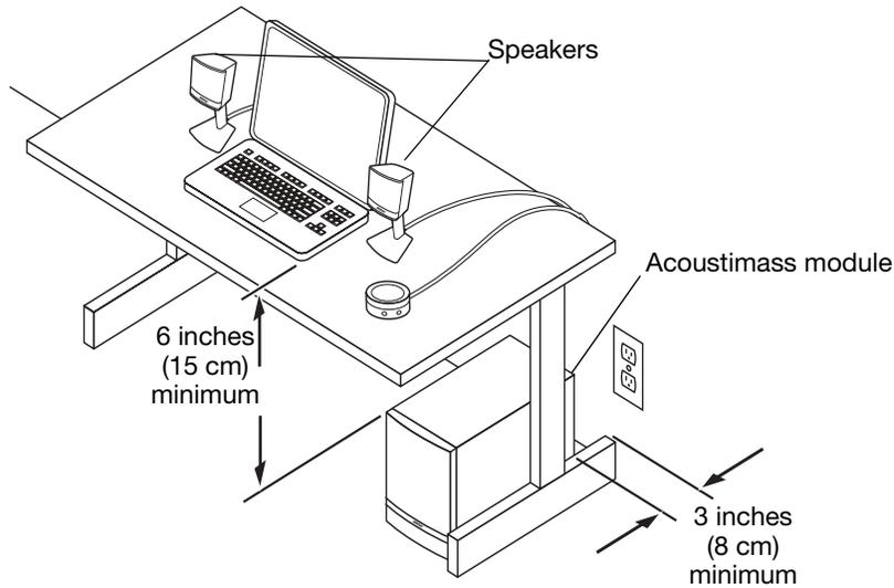
**Positioning the Acoustimass® module**
