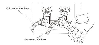
2. Connect the hot and cold water inlet hoses to the hot and cold water faucet.
