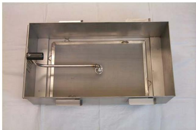
Filter leaf properly positioned in filter pan.
