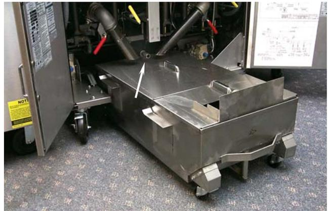
The filter pan slides under the fryer (above), connecting with a slip fitting (right). The slip fitting is located between the drain tubes (above, arrow).
