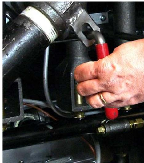
When the computer displays *FILL*, close the drain valve to begin refilling the frypot.
