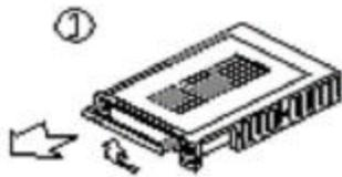
**Step 3: Unclip the release latch with the word "OPEN," printed beside it by gently pushing on the latch.**
