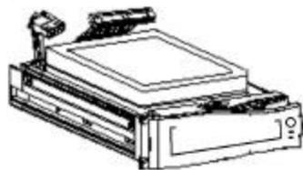
Take the Hard Disk Drive and connect the two cables from the back of the Cartridge Casing to the HDD.
