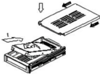
Reinsert the Cartridge Casing into the DXR109
