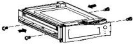
**Step 7: Slide the top Cover over the Cartridge Casing**
