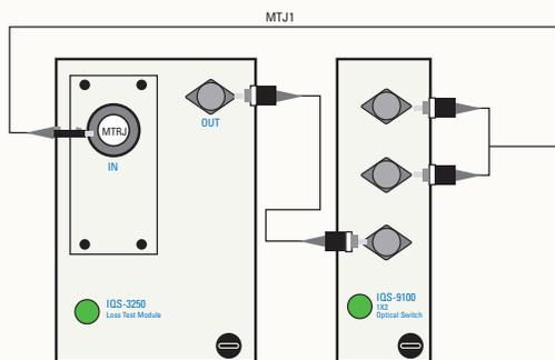
Basic configuration for testing multifiber connectors such as MTP and MT-RJ.
