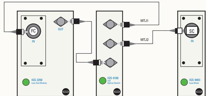
With an additional loss meter and a 1x2 optical switch, hybrid simplex assemblies can be efficiently tested. The two master test jumpers and detectors are configured for the different connectors of the hybrid assembly.
