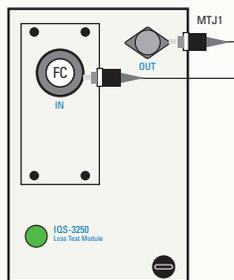
Basic configuration for testing simplex and multifiber bundles.
