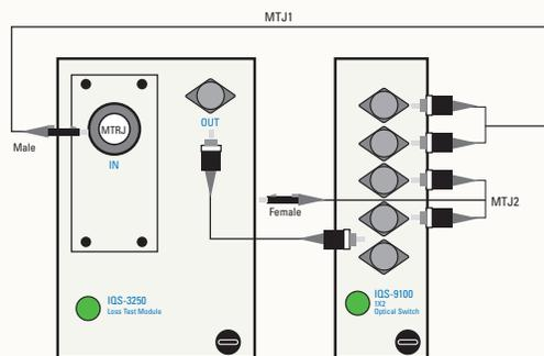
By doubling the number of switch ports, the system can be configured to accept both male and female multifiber connectors. The end result is faster and simpler testing in a single sequence.
