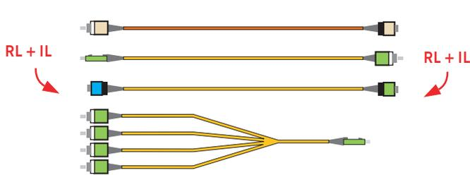
Simplex, duplex, multifiber and fanout, with or without hybrid connectors.
