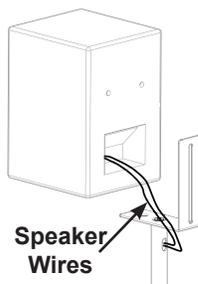
Open the EFB Package and remove the small Black Spacers and place them over the holes in the back of your speaker where the two plastic wall spacers were removed.
