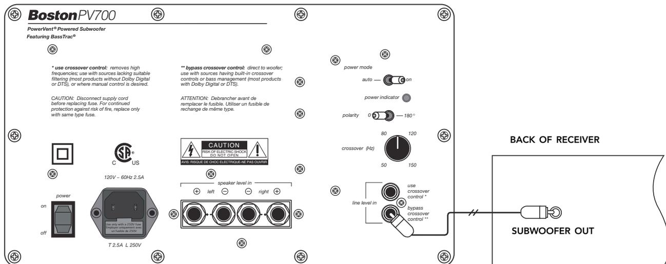
If you do not wish to run RCA cables to your subwoofer, you may use speaker wire to connect the subwoofer in parallel with your main speakers (see diagram below). The subwoofer does not present any additional load to your receiver.
