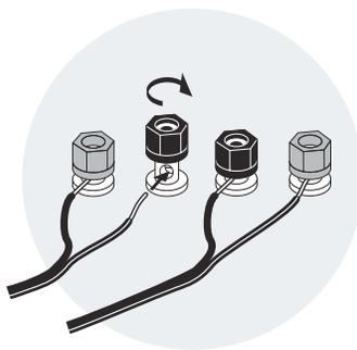
**Using the five-way binding posts:** The binding posts permit easy connection to banana plugs, spade lugs, and bare wire. Insert the wire in the hole (as shown on left) or a 3/8-inch spade lug over the post and tighten. For banana plugs, remove the red and black caps from the end-holes and insert either dual or single banana plugs (as shown on right).
