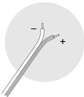
**IMPORTANT:** Typically, one side of the wire is smooth. Connect this side to the - (black) connection. The other side has a rib or stripe. Connect this to the + (red) connection.
