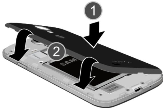
2. Press along the edge of the back cover (3) until you have a secure seal.
