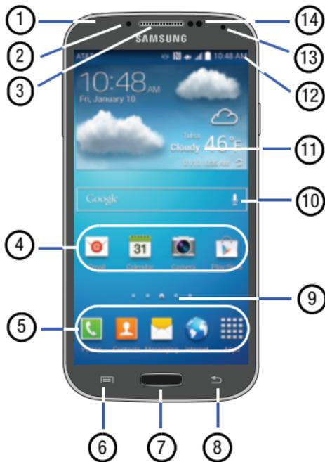
1. **Status light:** displays red when charging or the battery is low, blue when a notification has arrived or you are voice recording, and green when fully charged.
