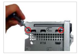
**Step 6.** Remove the indicated screws from the opposite side of the bracket and set aside.
