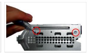
**Step 5.** Using the enclosed magnetic screwdriver, remove the two (2) indicated screws and set aside.
