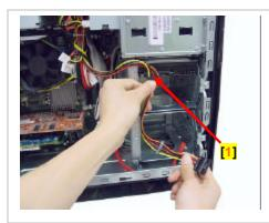
**Step 12.** Gently reconnect the previously removed power connector marked P8 [1] into the hard drive as indicated above.
