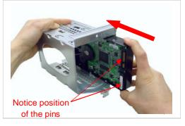
**Step 8.** Gently insert the new hard drive into the bracket in the direction of the arrow. Align the new drive in the same position as the original hard drive.
