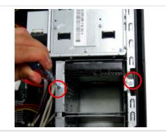
**Step 11.** Using the enclosed magnetic screwdriver, reinstall the two (2) previously removed screws. **IMPORTANT**! Do not over tighten the screws.
