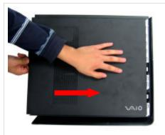
**Step 14.** Re-assemble the chassis panel cover. And reinstall the screws removed in step 1. Connect your PC and continue with the recovery following the instructions on the back of the recovery disk's case. Return the original hard drive to Sony following the included shipping instructions.
