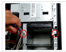
**Step 3.** Using the enclosed magnetic screwdriver, remove the two (2) indicated screws from the hard drive bracket.
