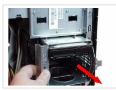
**Step 4.** Pull the hard drive bracket enclosure from the unit in the direction of the arrow.
