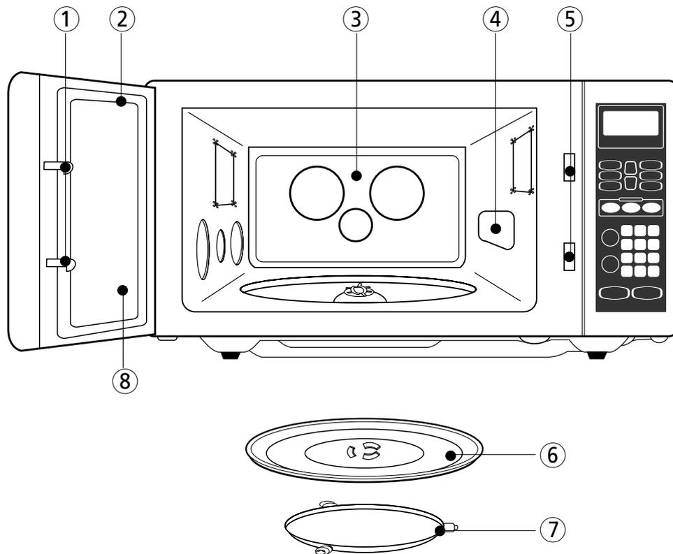
**1. Door latch**-When the door is closed it will automatically shut off. If the door is opened while the oven is operating, the magnetron will automatically shut off.
