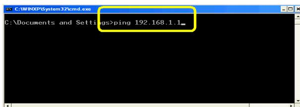
3. The Wireless Broadband Router shall reply and a similar screen as below is shown.
