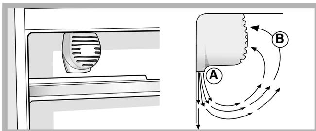
The A.I.R. System maintains a constant fridge temperature to keep food fresher for longer and will quickly restore the temperature to the correct level, even if the door is opened frequently: the blown air (A) is cooled when it comes into contact with the cold wall, whereas the hotter air (B) is sucked up (see *diagram*). The back wall may be covered in frost or droplets of water, depending on whether the compressor is in operation or whether it is paused.
