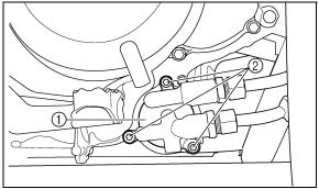
1. Engine oil filter cover 2. Engine oil filter cover bolt ( $\times$  3) 8-7
