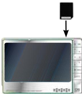
The memory card slot, located on top of the device, on the right side, allows you to insert one of the following cards (which are not supplied):
