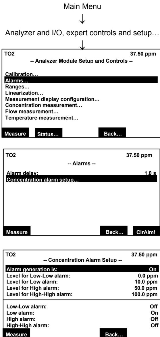
Move the cursor to the "Alarms..." line and press the  $\downarrow$  key. The "Alarms" menu will display as shown below.
