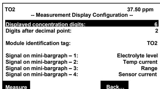
The first two lines allow for setting the concentration value displayed precision and number of digits.
