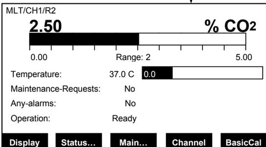
Continue pressing F4 to display the desired channel depending on the installed analyzer configuration, ultimately returning to the first channel.
