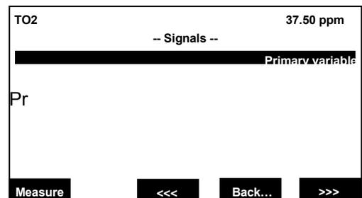
Press the F5 key to go to a further menu to choose the Primary Variable signal for the analog output. The Primary Variable is the actual oxygen concentration.
