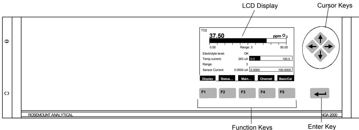
Figure 3-1. Platform Front Panel
