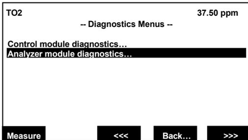
This menu has two submenus for viewing and resetting any software errors.
