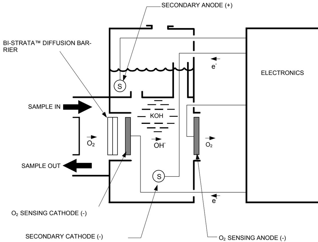
Figure 1-1. Trace Oxygen Detector Coulometric Principle
