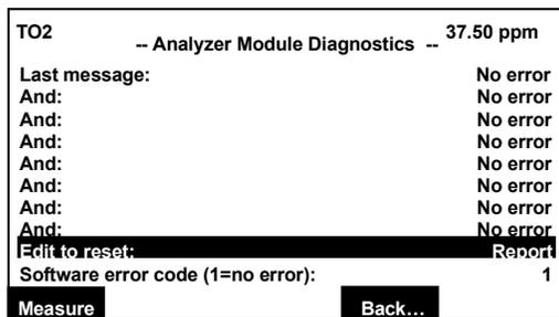
This menu displays any software error messages of the analyzer.
