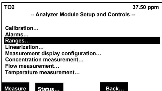
Move the cursor to the “Ranges...” line and press the  $\downarrow$  key. The “Ranges” menu will display as shown below.
