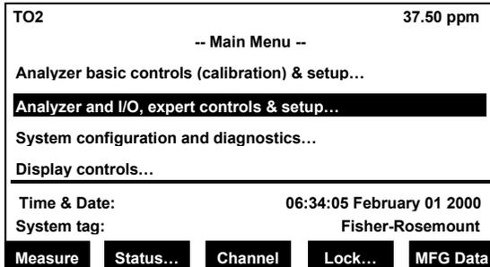
From the Main menu, move the cursor to the “Analyzer and I/O, expert controls & setup...” line and press the  $\downarrow$  key. The menu will display as shown below.
