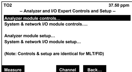
Select the “Analyzer module control...” line and press the  $\downarrow$  key. The “Analyzer Module Setup and Controls” menu will display as shown.
