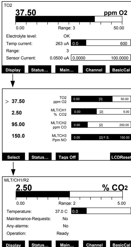
From the single channel display (Measure) press F1 (Display) to change to the Multi Component Display of all other installed Analyzer Modules.
