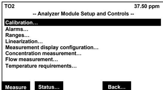
Note: Whenever the “Channel” tag appears above the F3 key, pressing F3 will switch to any other installed analyzer modules, one after the other and eventually back to the TO2 module. When activating any other installed module, the menus will be different depending on that module. See each module’s manual for a description of those menus.
