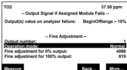
Normal: The absolute measurement signal will be sent to the analog output.
