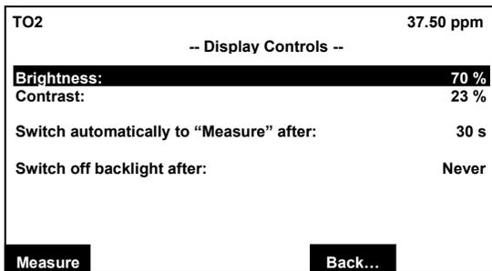
These values can be reset to the defaults from the Multi Channel display screen (F1 from the "Measure" screen) by pressing F5 (LCDReset). It can also be reset from the startup screen by pressing F1 (see Figure 3-8).
