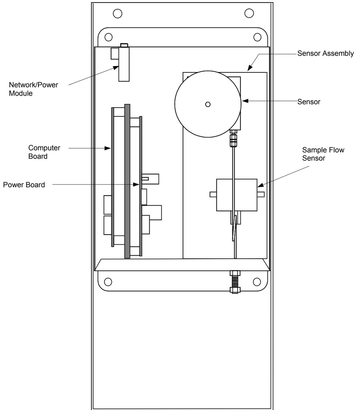
Figure 1-2. Trace Oxygen Analyzer Module - Top View
