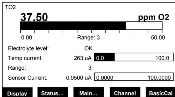
Figure 3-5. Measure Mode Display
