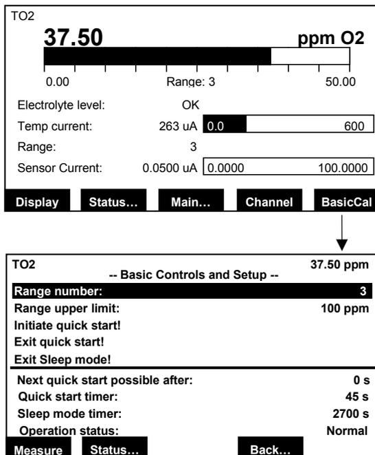
From the Measure menu press the F5 key (BasicCal) to reach the "Basic Controls and Setup" menu.
