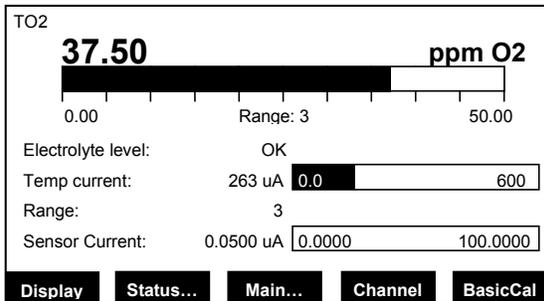
Press F4 (Channel) to change to the Single Component Display of any other installed Analyzer Modules.
