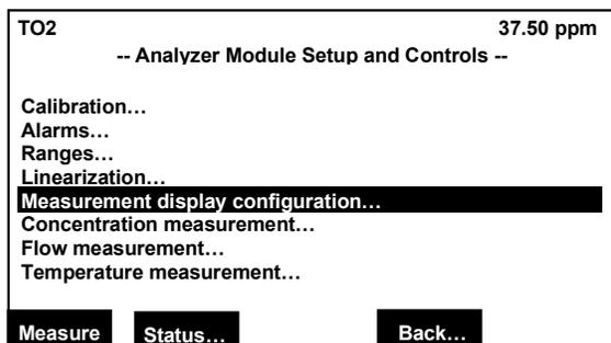
Move the cursor to the “Measurement display configuration...” line and press the  $\downarrow$  key. The “Measurement Display Configuration” menu will be displayed.
