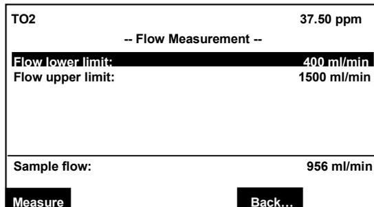
Set the upper and lower alarm limits for sample flow as desired.
