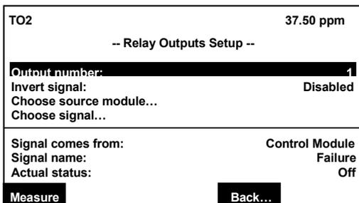
Select the “Configuration of relay outputs...” line in the “Local SIO Configuration Parameters” menu to change to the submenu “Relay Output Setup” to attach signals to the relay outputs.
