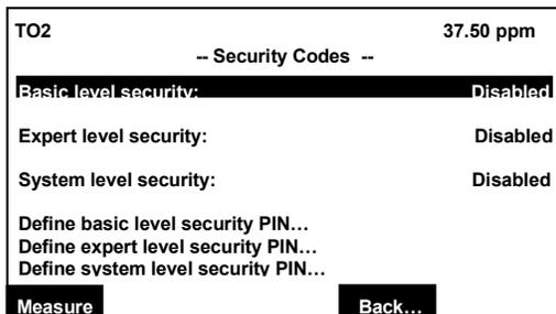
This menu is used to set the security codes for the three levels of security.
