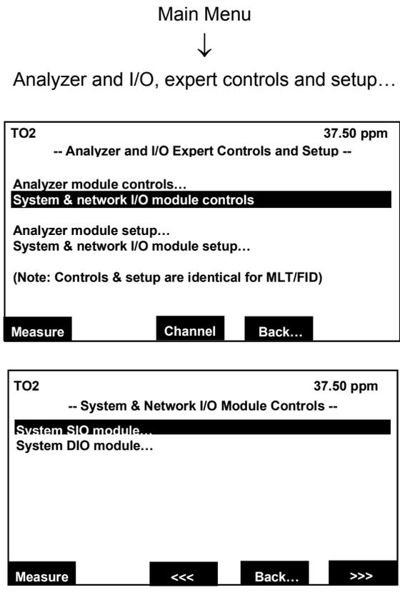
Press the ↓ or → keys to change to the desired submenu.
