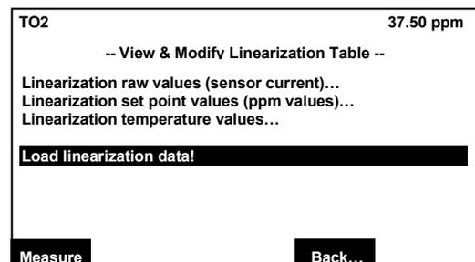
Select Load linearization data! press enter. The new data is now loaded into the analyzer and accurate measurements can be obtained.
