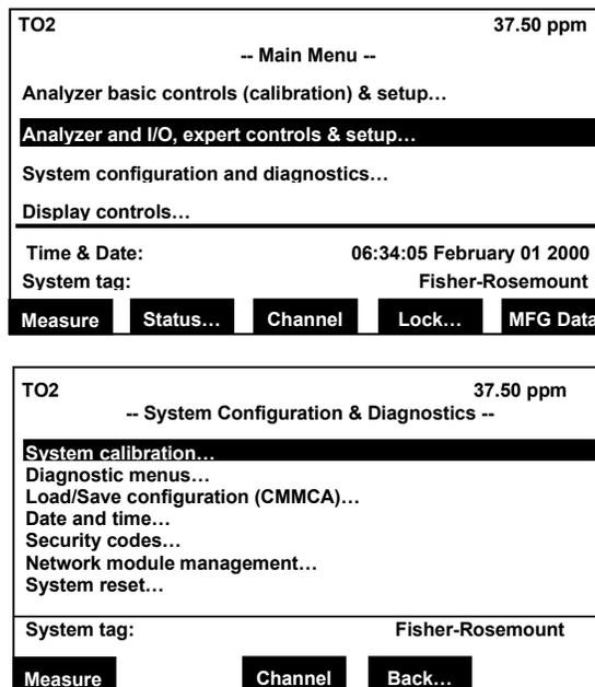
**Figure 3-26. System Configuration and Diagnostics**
