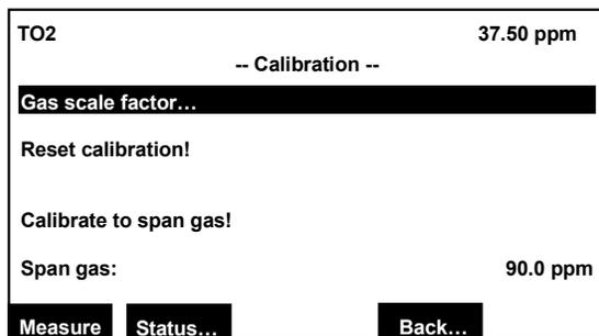
Move the cursor to the “Gas scale factor...” line and press the  $\downarrow$  key. The “Gas Scale Factor 1/0” menu will display as shown on the next page.
