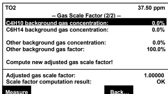
To view and adjust additional background gas components, press the F5 key to display the second menu.
