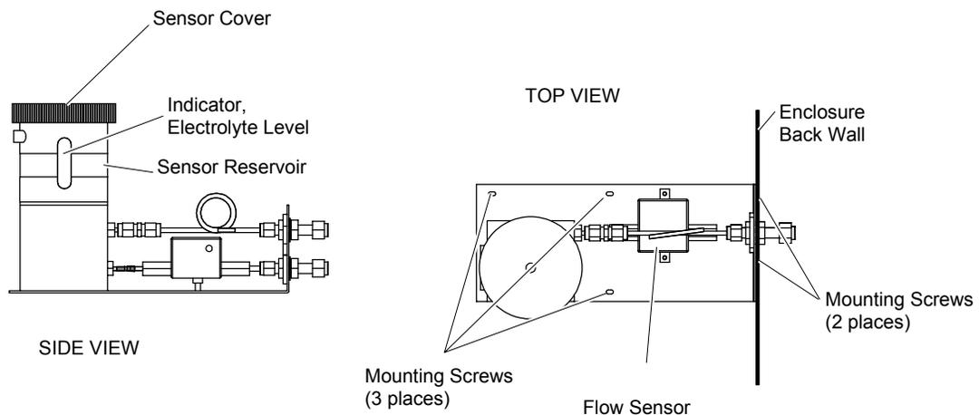
**Figure 4-1. Sensor Assembly**
