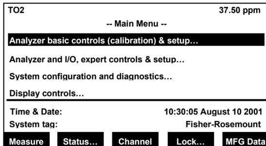
From the Main Menu, move the cursor to Analyzer basic controls (calibration) & setup...
