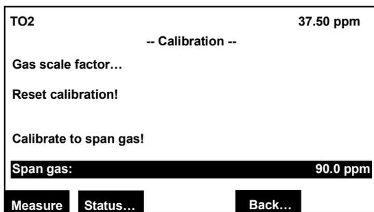
Move the cursor to the "Calibrate to span gas!" line and press the  $\downarrow$  key. The new span calibration will be calculated.
