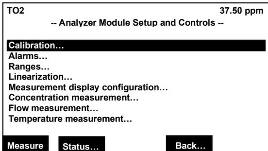
Move the cursor to the “Calibration...” line and press the  $\downarrow$  key. The “Calibration” menu will display as shown below.
