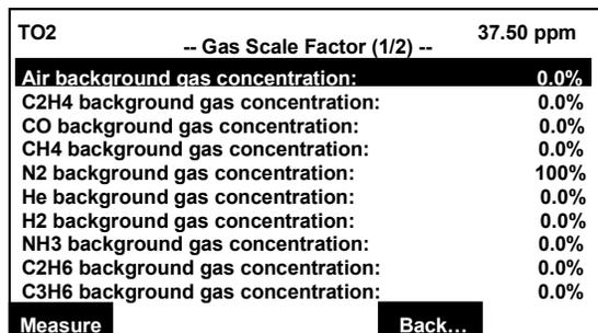
Enter the volumetric percentages of each component present in the sample gas.
