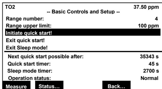
In the Basic controls and Setup menu, move the cursor to the "Initiate quick start!" line and press the  $\downarrow$  key. The analyzer will begin the quick start function immediately. This process will take about 45 seconds. The "Quick start timer" will count down this period.
