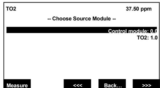
Choose desired source module for the relay output number (1-3) being configured.
