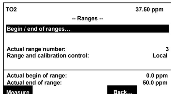
The “Actual range number:” line on the Ranges menu shows the current range number being used and allows changing of the range. The range values display below the line.
