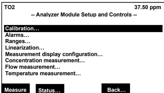
Introduce a suitable span gas to the analyzer and allow the reading to stabilize.
