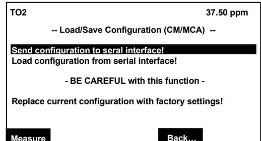
This menu provides several functions to send or load configuration data of the analyzer through the serial interface. These functions are only available if an SIO with serial interface is installed.
