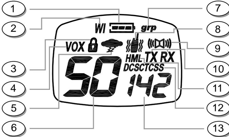
1. **BATTERY METER** – Indicates the battery level.
