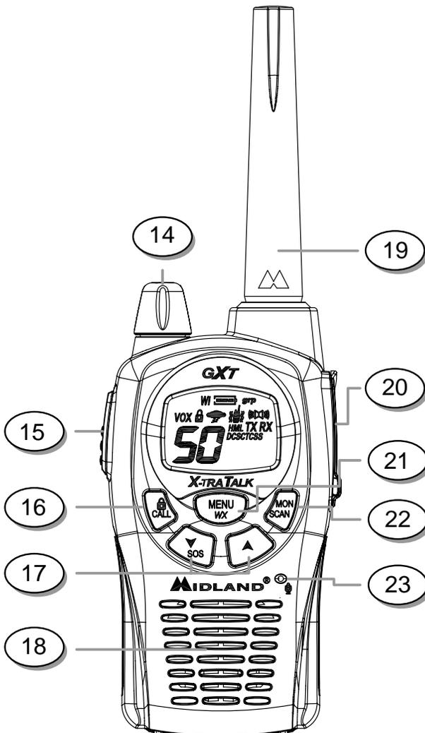
14. **POWER/VOLUME KNOB** – Turn clockwise to turn the power on and increase the volume level. Turn counter-clockwise to decrease the volume level and turn the power off.
