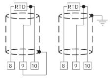
Fig. 5 RTD INPUT WIRING
