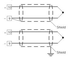
Fig. 4 THERMOCOUPLE INPUT WIRING
