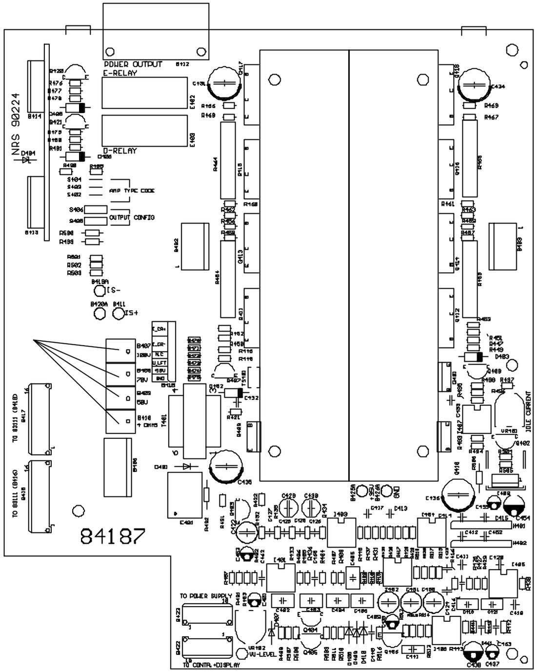
figure 8 printed board assembly 84187 in the DPA 4120 showing the NRS 90224 pilot tone & ground fault surveillance and the bridges B411 and S405, S406 for switching the output voltage; inserted
