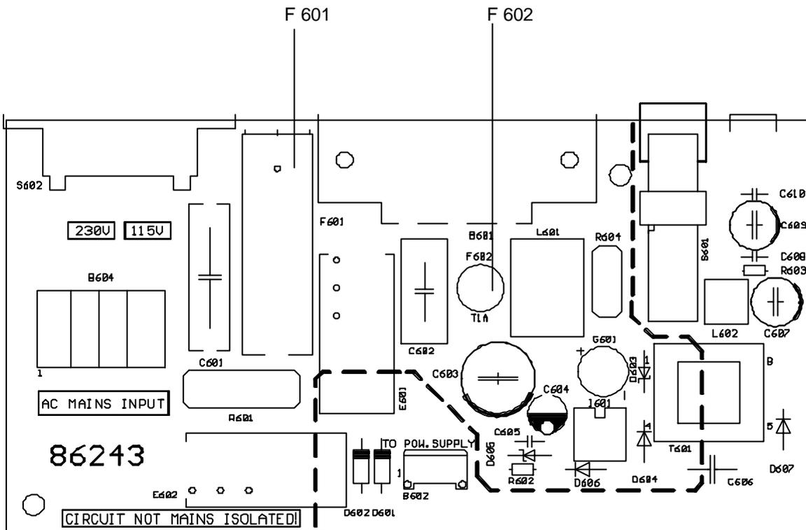
figure 12 printed board assemblies 86243 DPA 4120 and DPA 4140 showing the AC fuses F601 and F602
