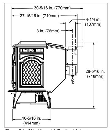
Figure 7.4 - Side View with Top Vent Adapter
