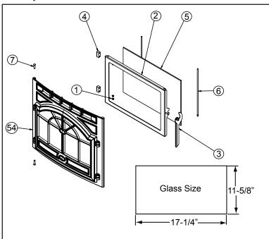
Figure 37.1 - Door, Face, Glass & Door Latch Assembly
