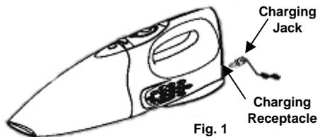
4. The normal full charging time for this vacuum is 20 hours. The vacuum cleaner will run for maximum operational time only if it has been fully charged. To fully charge the unit, run the vacuum cleaner until it stops, then fully recharge the battery.
