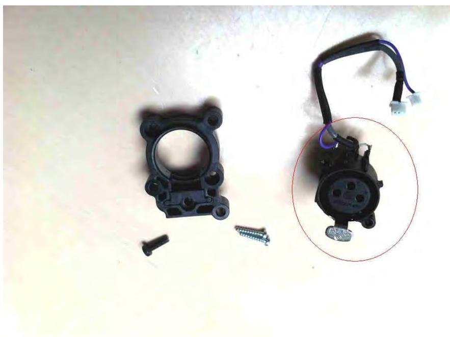
Separate the connector section from the XLR chassis
