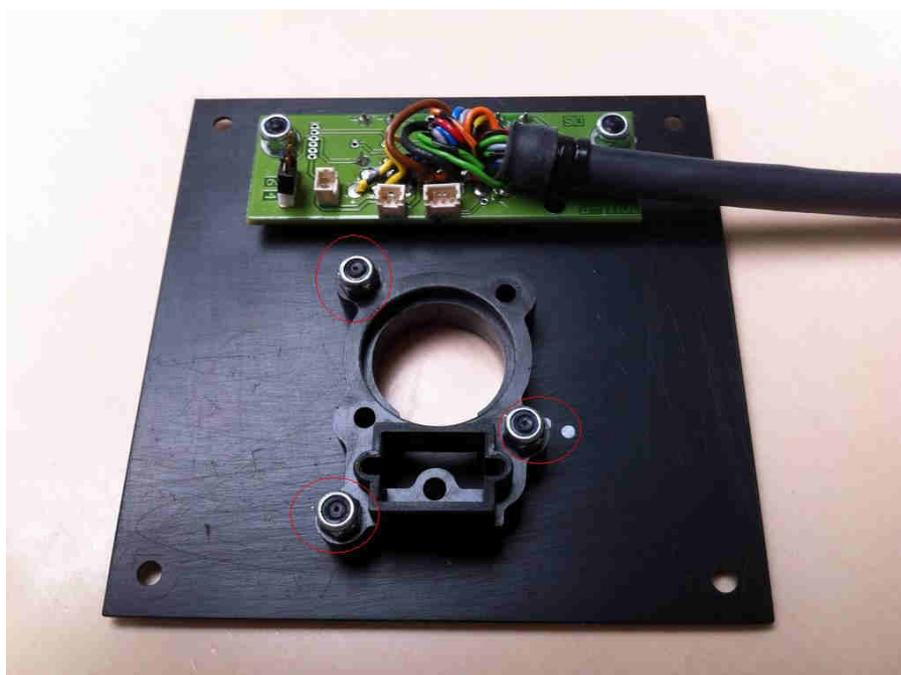
Fasten the XLR chassis to the from plate with the 3 M3 nuts.
