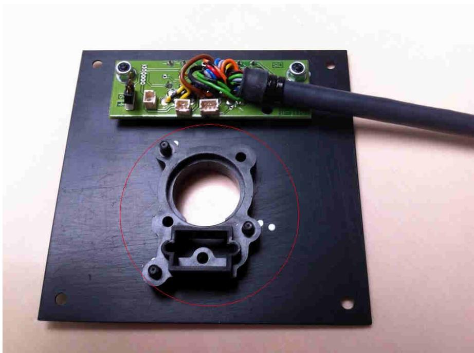
Put the XLR chassis back onto the front plate
