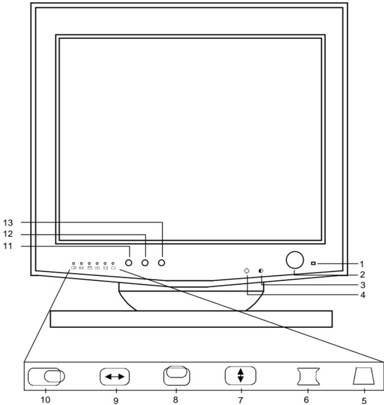
1. **POWER LED:** Lit when monitor is ON. Unlit when monitor is OFF.
