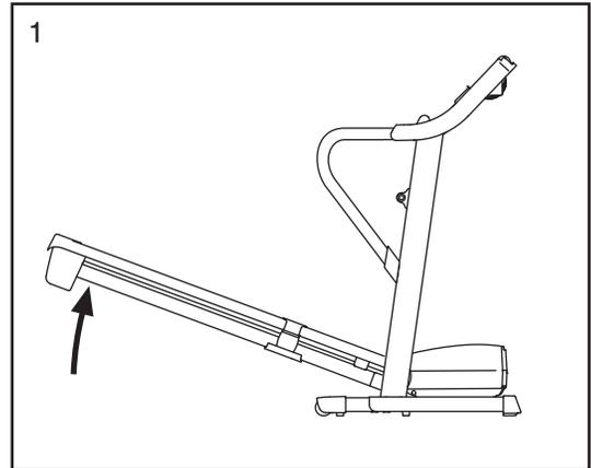
2. Move your right hand to the position shown, and hold the treadmill firmly. Using your left hand, pull the latch knob to the left and hold it. Raise the frame until the catch is past the latch pin. Then, slowly release the latch knob. **Make sure that the frame is securely held by the latch pin.**
