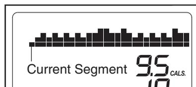
profile represents the current segment of the workout. The height of the flashing segment indicates the speed setting for the current segment. At the end of each segment, a series of tones will sound and the new speed setting, new incline setting, and the next segment of the profile will flash in the display.
