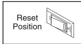
**IMPORTANT:** The console features a display demo mode, designed to be used if the treadmill is displayed in a store. If the displays light as soon as you plug in the power cord and switch the reset/off circuit breaker to the reset position, the demo mode is turned on. To turn off the demo mode, hold down the Stop button for a few seconds. If the displays remain lit, see THE INFORMATION MODE on page 17 to turn off the demo mode.
