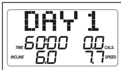
Programs button. When the pound-a-week workout is selected, the words "A Pound A Week" will appear in the display, followed by "Day 1," "Day 2," "Day 3," "Day 4," or "Day 5." In addition, the maximum incline setting of the workout and the maximum speed setting of the workout will flash in the display. A few seconds after the pound-a-week workout is selected, a profile of the speed settings of the workout will scroll across the display.
