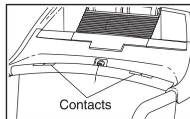
To measure your heart rate, **stand on the foot rails** and hold the metal contacts on the handrail—**avoid moving your hands**. When your pulse is detected, a heart-shaped indicator will flash in the right side of the display each time your heart beats, one or two dashes will appear, and then your heart rate will be shown. **For the most accurate heart rate reading, continue to hold the contacts for about 15 seconds.**
