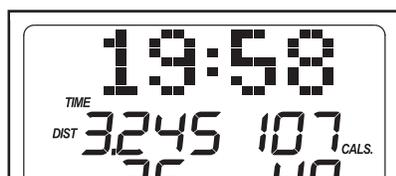
The left side of the display can show the elapsed time, the distance that you have walked or run, the approximate number of grams of carbs that you have burned, and the incline level of the treadmill. Note: When a workout is selected, the display will show the time remaining in the workout instead of the elapsed time.
