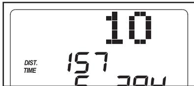
The center of the display will show the number of hours that the treadmill has been operated. The lower right corner of the display will show the total number of miles or kilometers that the walking belt has moved.
