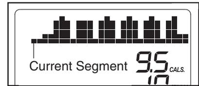
The workout will continue in this way until the last segment of the profile flashes in the right display and the last segment ends. The walking belt will then slow to a stop.
