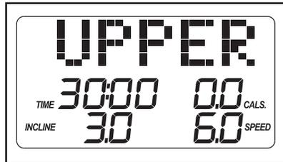
Programs button repeatedly. When a cross training workout is selected, the display will show the word UPPER, LOWER, or TOTAL and the workout duration. In addition, the maximum incline setting of the workout and the maximum speed setting of the workout will flash in the display. A few seconds after a cross training workout is selected, a profile of the speed settings of the workout will scroll across the display.
