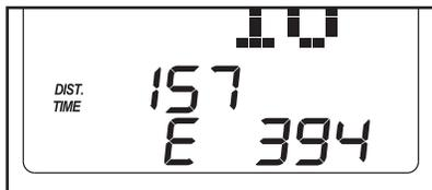
In addition, an "E" for English miles or an "M" for metric kilometers will appear in the lower left part of the display. To change the system of measurement, press the Speed increase button.
