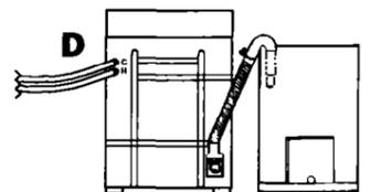
If a longer drain hose is needed, drain hose extension kit (Part No. 285702) is available from authorized parts distributors. If drain hose must be shortened, use hose kit (Part No. 285442).
