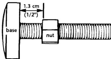
**11.** Screw nut down on legs to within 1.3 cm (1/2 inch) of base.
