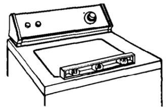
**14.** Tilt washer forward, raising back legs 2.5 cm (1 inch) off of floor to adjust rear self-leveling legs. Gently lower washer to floor. Check levelness of the washer by placing a carpenter's level on top of the washer, first side to side; then front to back.
