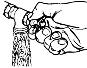
**7.** Run water through both faucets into a bucket to get rid of particles in the water lines that might clog hoses. Mark the hot water faucet.
