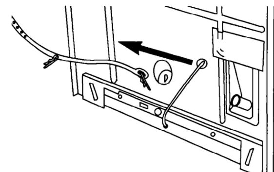
**Pull the strap completely out of the washer.**
