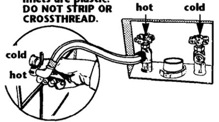
**9.** Attach bottom hose (inlet marked "H") to hot water faucet. Attach top hose (inlet marked "C") to cold water faucet. Adapters may be necessary to connect the hoses to the faucets. Tighten couplings to faucets. **DO NOT OVERTIGHTEN;** this could cause damage to couplings.
