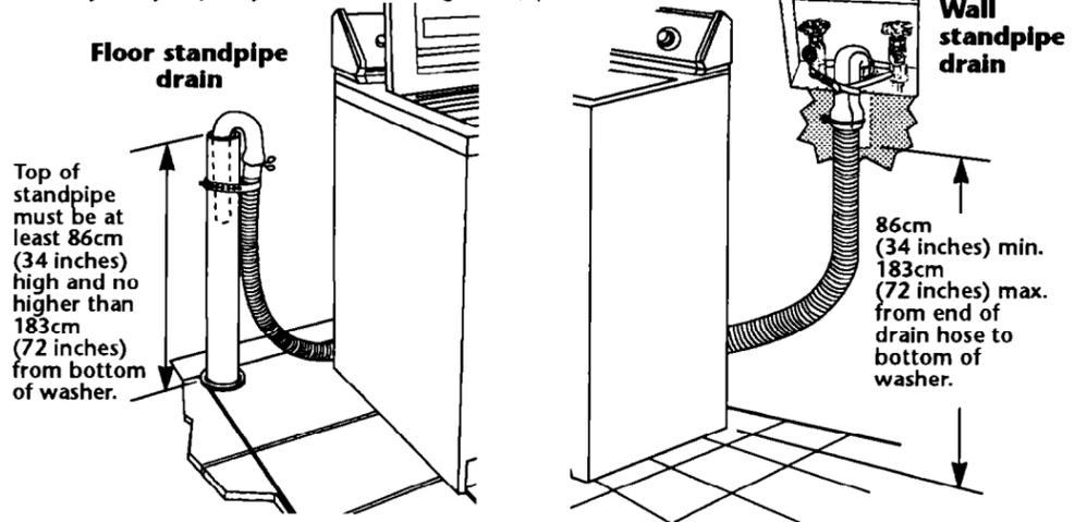
If a longer drain hose is needed, use drain hose extension kit (Part No. 285702). If drain hose must be shortened, use kit (Part No. 285442). Both kits are available from Whirlpool-authorized parts distributors.
