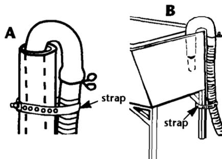
Put "hook" end of drain hose in laundry tub or standpipe. Tightly wrap the shipping strap around the drain hose and laundry tub or standpipe or inlet hose as shown in Figures A-B. Push plug into the nearest hole in the shipping strap.
