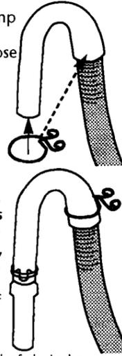
If drain hose does not fit into standpipe or is being placed over the edge of a laundry tub, open other hose clamp with pliers and place clamp over rigid end of drain hose.
