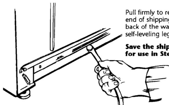
Pull firmly to remove the other end of shipping strap from the back of the washer to release self-leveling legs.
