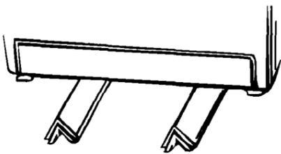
**10.** Stack two corner posts on top of each other. Tilt washer backwards and insert corner posts 7.6 cm (3 inches) from one side of washer as shown. Repeat with other corner posts on other side of washer.
