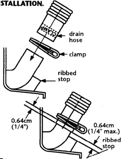
**5.** To prevent the drain hose from coming off or leaking, it must be installed per the following instructions.
