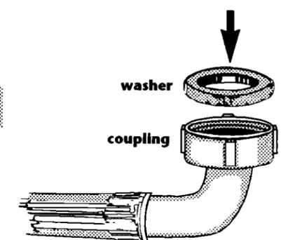
3. Insert a flat washer into **each** end of the inlet hoses. Check that washers are firmly seated in couplings.
