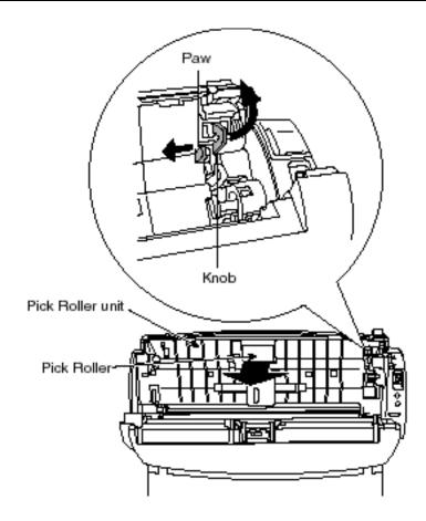
5) When mounting a new pick roller unit, insert it so that the pick roller unit paw slides into the pick roller unit hole of the equipment.
