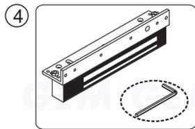
4 Use the Allen wrench to tighten the screws into the L bracket.
