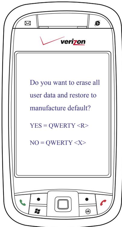
3. Slide open the hardware keyboard, then press **R** to do a hard reset.
