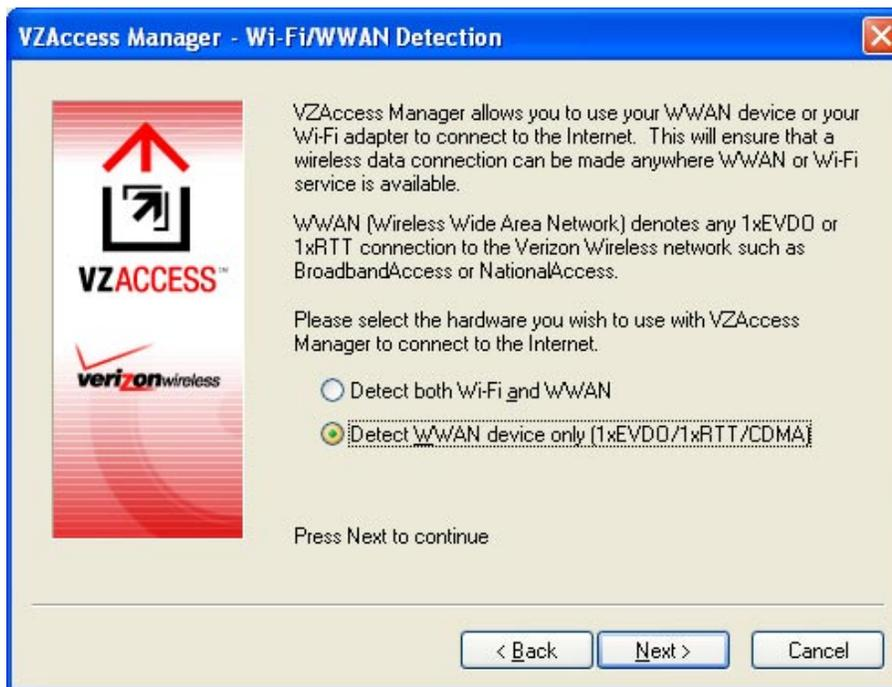
**Note** If your computer has built-in Wi-Fi or has a Wi-Fi card installed, you can select the **Detect both Wi-Fi and WWAN** option. This allows you to use either your XV6800 or your computer's Wi-Fi adapter to connect your notebook to the Internet. For more information, refer to the VZAccess Manager documentation on the CD.
