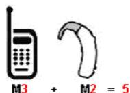
In the above example, if a hearing aid meets the M2 level rating and the wireless phone meets the M3 level rating, the sum of the two values equal M5. This should provide the hearing aid user with "normal usage" while using their hearing aid with the particular wireless phone. "Normal usage" in this context is defined as signal quality that is acceptable for normal operation.
