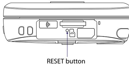
You can also perform a hard reset (also known as a full reset). A hard reset should be performed only if a soft reset does not solve a system problem. After a hard reset, the device is restored to its default settings — the way it was when you first purchased it and turned it on. Any programs you installed, data you entered, and settings you customized on your device will be lost. Only Windows Mobile software and other pre-installed programs will remain.
