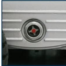
2. Use the oil supplied to fill the crank case until the oil level as seen in the oil sight glass (16) is up to the mid point of the red circle.
