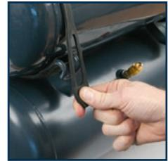
**WARNING.** When extending the rubber straps be careful. If released early they can flick back and hurt you. Make sure that your face is at a safe distance from the rubber straps while they are being stretched.
