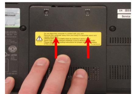
**Step 19.** Re-attach the Hard Drive Door by sliding it towards the unit.
