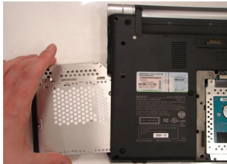
**Step 8.** Carefully remove the ODD from the unit.
