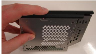
**Step 13.** Align the tabs on the bezel with the tab holes located on the ODD. Carefully press the bezel into place.
