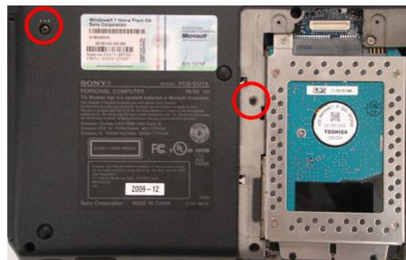
**Step 18.** Reinstall the two (2) ODD Bay screws to secure the ODD.
