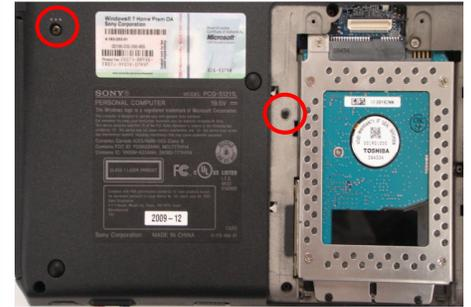
**Step 6.** Using the enclosed magnetic screwdriver, remove the (2) screws securing the ODD Bay. **Put aside the ODD Bay screws for later in the procedure.**
