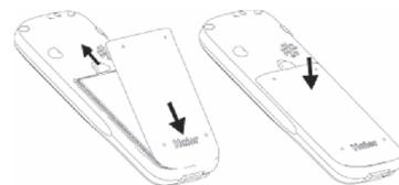
Installing the battery
