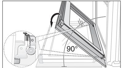
4. Fold up the clamping levers (A) on both door hinges back into their original positions.
