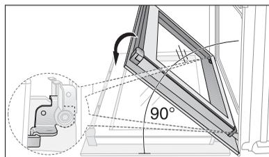
2. Undo the clamping levers (A) on both door hinges **fully**.
