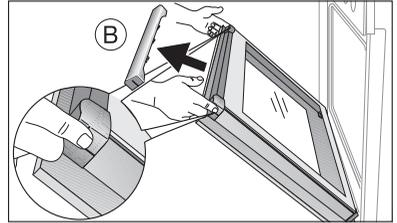
5. Take hold of the door glass on its upper edge and take it out of the guide by pulling it upwards.
