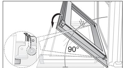
3. Fold up the clamping levers (A) on both door hinges back into their original positions.
