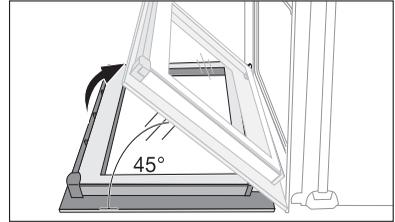
4. Take hold of the oven door with a hand on each side and pull it away from the oven at an upwards angle (**Take care:** It is heavy).
