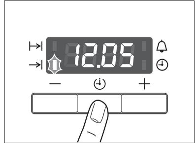
2. Using the  $+$  or  $-$  button set the desired switch-off time.
