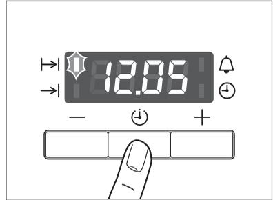
2. Using the  $+$  or  $-$  button set the desired cooking time.
