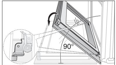
2. Undo the **clamping levers (A)** on both door hinges **fully**.
