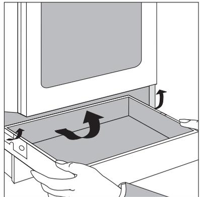
3. When re-inserting the drawer, make sure that the pan drawer's middle guide engages into the middle guide rails.
