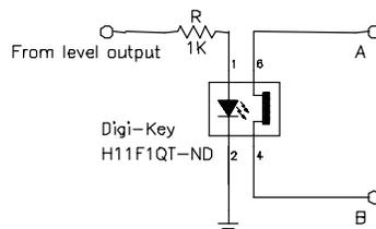
This is a simple, yet useful way of isolating the URC1 from the unit being controlled. This setup will work well for any circuit (within current limits) that requires a variable resistance. For example this can be used to control a form of squelch on a radio called level detection. This simple circuit can be used in
