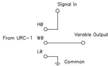
This is the simplest way of controlling signal levels such as volumes, voltages, powers, etc. Always tie the common ground of the URC1 to the common on the unit you are trying to control. If you are worried about the common on the unit to be controlled not being isolated, run the URC1 off of an isolated power supply. Using this method should protect the URC1 from damage from grounding errors. L0 does not have to be tied to common, but must not go lower in voltage than the common of your URC1.
