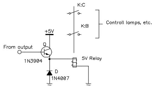
Once connected to the relay, the URC1 can turn a number of devices on and off, such as home security systems, lights, answering machine, lawn watering system, swimming pool filters, etc. Be sure the coil on the relay has a resistance of no less than 100 ohms to be safe. If it is less, use a transistor with a higher power dissipation rating.
