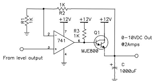
This configuration allows a user to adjust a 12VDC-18VDC unregulated power supply to a 0-10VDC regulated supply. The regulation in this case is limited to how well the URC1's regulator is operating. Parts can be modified in value to
