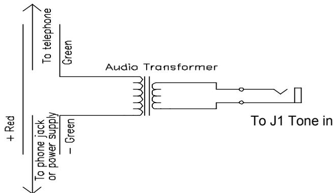
This is how you are able to insert the confirmation tones into the telephone line so that when you are dialing from a remote location you can hear the URC1 talk back to you, and let you know that a code was correctly received and processed. You may also receive tones as well with this circuit. Notice it is in parallel with the phone line instead of series like the previous circuit.
