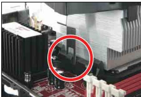
5. On the other side, push the retention clip straight down to lock into the plastic lug on the retention frame.
