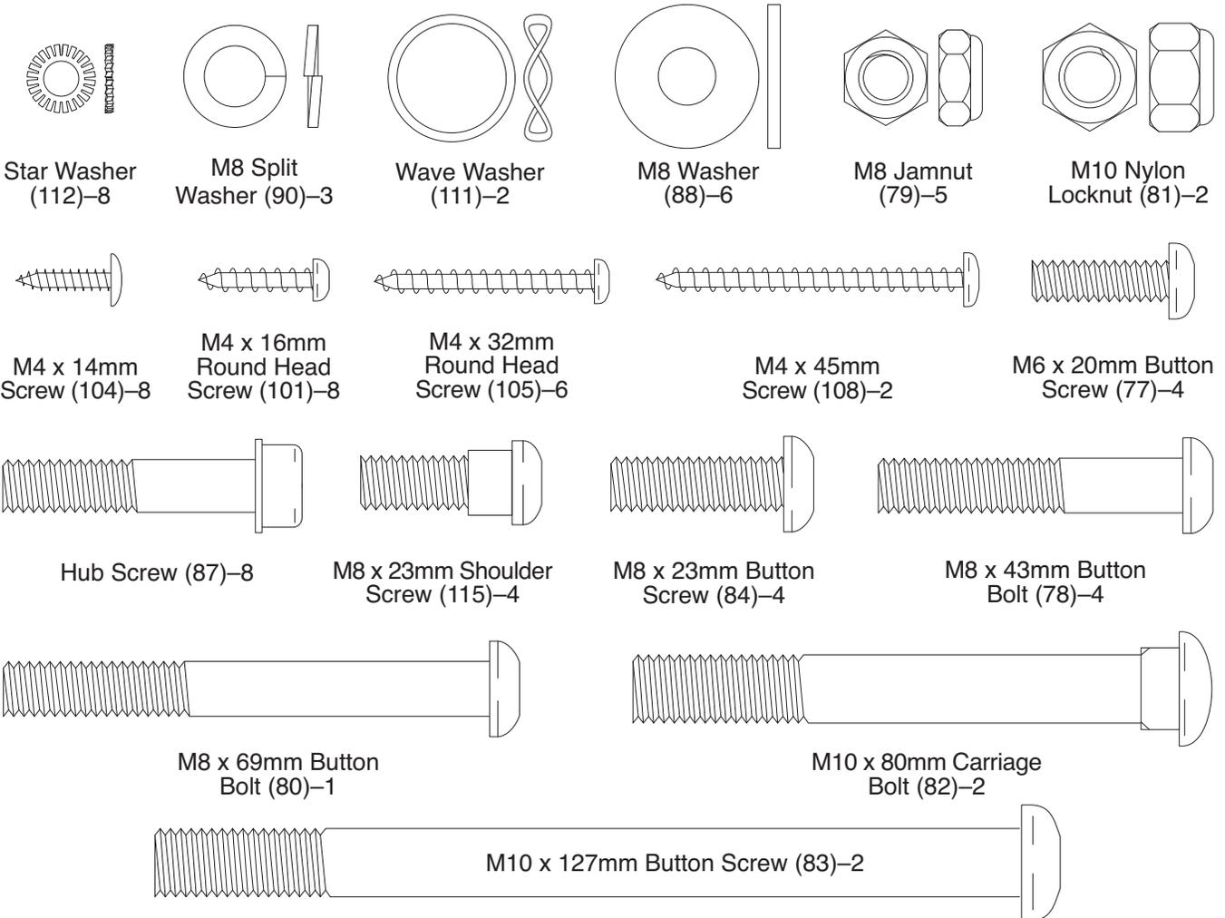
1. While another person lifts the Base (1), attach the Front Stabilizer (6) to the Base with two M10 x 80mm Carriage Bolts (82) and two M10 Nylon Locknuts (81).
