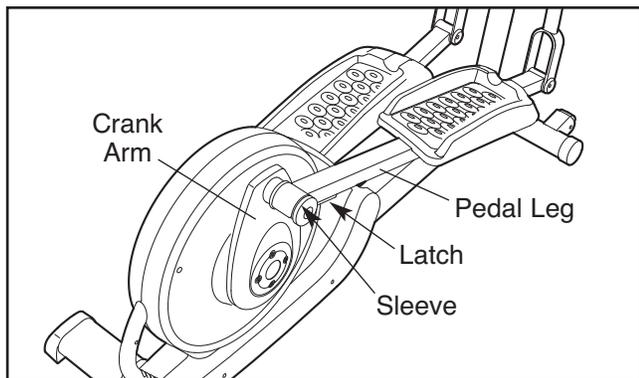
Next, raise the pedal legs until they touch the magnets on the upper body arms; the magnets will hold the pedal legs in place. Then, hold the handle and lift the frame until it locks in a vertical position.
