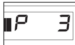
If pulse control program 3 is selected, a profile of the target heart rate settings of the program will scroll across the center of the display.
