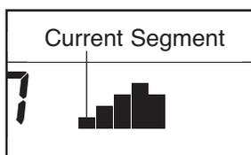
When only three seconds remain in the first segment of the program, both the Current Segment column and the column to the right will flash, a series of tones will sound, and *all target heart rate settings will move one column to the left*. The target heart rate setting for the second segment will then be shown in the flashing Current Segment column.
