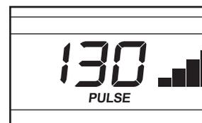
If pulse control program 4 is selected, the target heart rate setting for the program will flash in the display. If desired, press the Resistance increase and decrease buttons to change the target heart rate setting (see **EXERCISE INTENSITY** on page 24).
