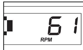
(revolutions per minute [rpm]). Note: When the distance program is selected, the display will show the number of revolutions still to be pedaled instead of the number of revolutions you have pedaled.
