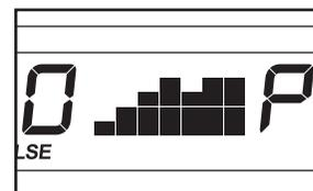
If pulse control program 4 is selected, a pulse symbol will appear in the center of the display. Each time a heartbeat is detected while you are using the handgrip pulse sensor, the pulse symbol will reappear.
